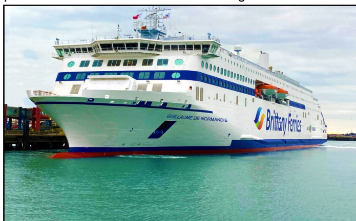
Guillaume de Normandie is hybrid fuelled on cleaner liquefied natural gas and battery. It can carry 1310 passengers.
